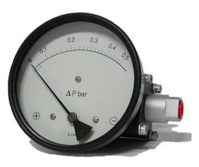
Differential Pressure Plus, Inc. Supplies quality differential pressure instruments designed to measure the difference in pressure between two points in a system and show it on a single dial instrument. A magnetic movement senses the differential pressure. The instrument has separate pressure and indicating chambers.
