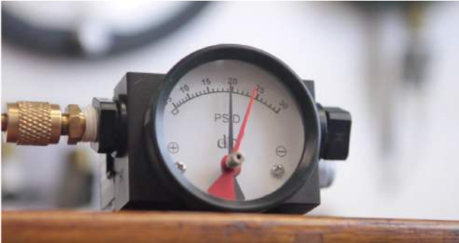
Follower Pointer: Shows Max Reading
