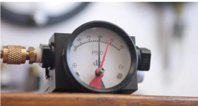
Follower Pointer: Shows Max Reading
